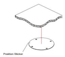
Apply the position sticker to the desired camera mounting position.
