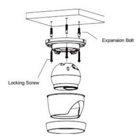
Fix the pedestal by drilling locking holes around the sticker and inserting three expansion bolts into the holes and fastening it with three locking screws.
