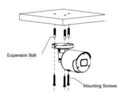
Insert three expansion bolts in place into the ceiling and fix the equipment with three mounting screws.
