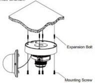
Use the position indicated on the position sticker to drill the holes needed to mount the camera base. Insert the expansion bolt into the holes. Match the base's mount openings to the expansion bolts position, then place the mounting screws through the base's mount opening into the expansion bolt. Tighten the mounting screws to ensure the camera base mounted securely.
